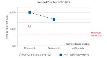
**Figure 1:** Notched Pipe Test according to ISO 13479 with varying notch depth. Test covered 110 mm SDR11 pipes with varied notch depth tested in hydrostatic pressure test at 920 kPa/80°C.
